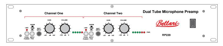
The RP220 provides clear sonic quality and performance for the working musician, studio operator or anyone who needs a preamp with the warm, smooth, analog sound. Each channel utilizes one premium 7025 tube in a unique configuration to give smooth controllable gain through transformer balanced inputs. The unit has both XLR and 1/4" inputs and outputs with a 30 dB Pad and a Phase Reversal switches to adapt to any performing or studio situation.
