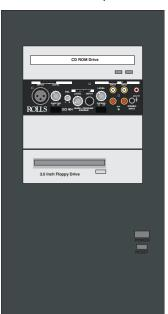
Select the drive bay you wish to mount the GCi404 into. Remember that you will have cords hanging down from the unit, so below a CD Rom drive is recommended. Remove the drive bay cover and gain access to the inside of your computer.
