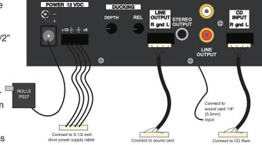
sound-card Input via a stereo Tip-Ring-Sleeve 1/8" (3.5mm) cable.
