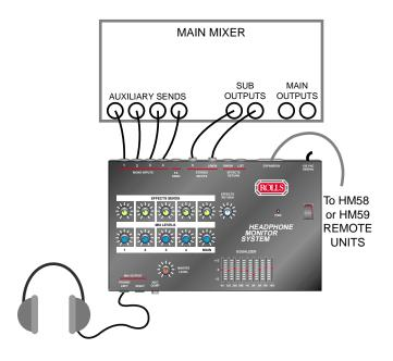
Shown below is an example for proper connection to a signal processor.
