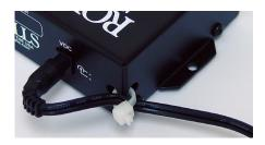
The holes in the back and side of the PA202 are for the attachment of a zip tie (not included). For power cord strain relief as needed.
