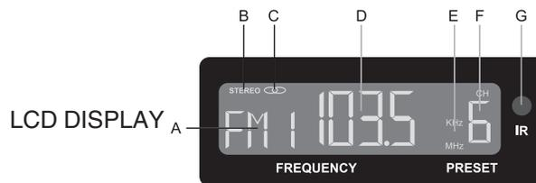
A: Band indicator and number. There are three banks of FM and two banks of AM presets. *NOTE: If the rear panel Frequency Select switch is set for 9kHz, the band will indicate MW 1 and MW2 instead of AM1 and AM2.*
